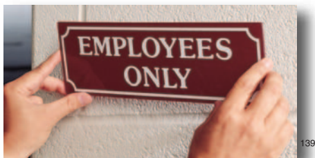
3M™ Double Coated Urethane Foam Tapes bond plastic signs to painted cinder block. The foam fills gaps between irregular surfaces. Various foam thicknesses are available for surface conformance based on the degree of roughness.
