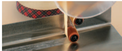
181 Save time and effort with the Scotch® ATG Adhesive System. You apply a precise strip of adhesive at the same time as the liner rewinds into the applicator.
