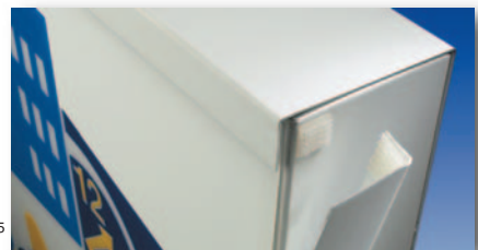
Die-cut 3M™ Scotchmate™ Reclosable Fasteners secure metal edge molding around an internally-illuminated sign. The molding holds the sign face in place and is readily removed for bulb replacement.
