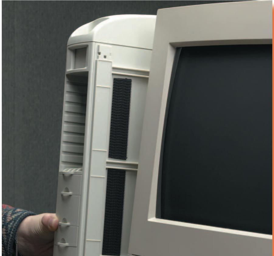
Removable plastic storage box for computer media attaches to the side of the CRT screen with strips of 3M™ Dual Lock™ Reclosable Fastener. Pressure sensitive adhesive backing bonds to many plastics on contact.
