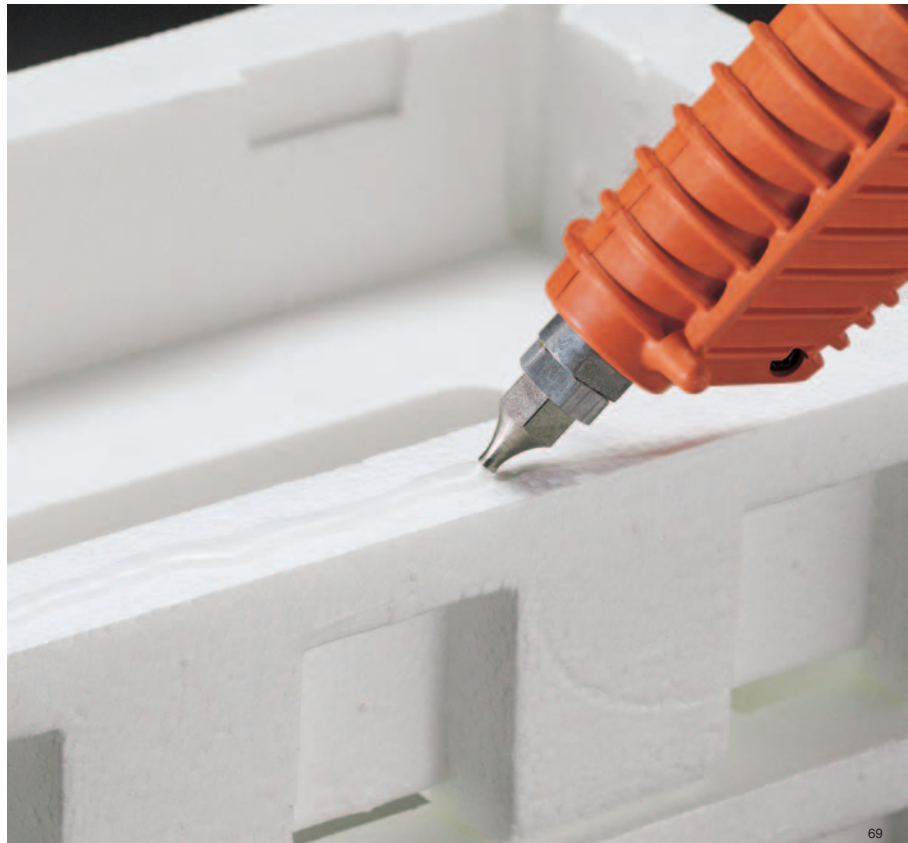
3M™ Scotch-Weld™ Hot Melt Applicator EC can be used with 3M low temperature (265°F/129°C) adhesive to effectively bond heat-sensitive substrates such as styrene foam.
