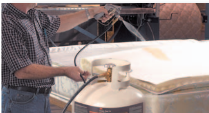
With 3M™ FoamFast Cylinder 74 Spray Adhesive a fast light coat bonds quilted fabric to solid core mattress. High coverage reduces applied cost. Foam-tearing strength prevents cover spin.
