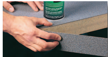
3M™ Hi-Strength 90 Spray Adhesive typically bonds edge banding in 60 seconds compared to 15-20 minutes for many typical bulk contact adhesives. Strength increases to an ultimate 230 psi in shear and 25 piw in peel.
