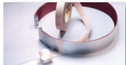
The silicone adhesive side of 3M™ Double Coated Tape 9731 bonds a silicone rubber insulator. The acrylic adhesive side adheres to the metal band. The band mounts to a wall bracket in industrial equipment.
